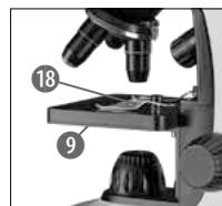
Now place the prepared specimen (18) directly under the objective on the microscope stage. The object should be located directly over the illumination (10).
