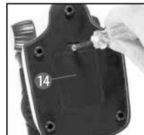
In the base of the microscope there is a battery compartment (14). Loosen the screw at the battery compartment cover with a small Philips screwdriver and remove the cover.
