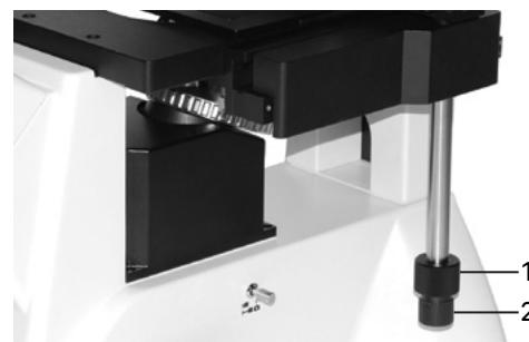
Fig. 13. Moving the specimen holder
