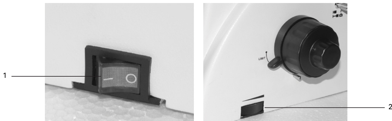
Fig. 5. Switching on the illumination and adjusting the brightness
