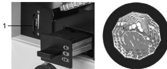
Fig. 26. Adjusting the field diaphragm
