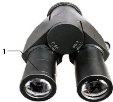
Fig. 10. Adjusting the diopter
