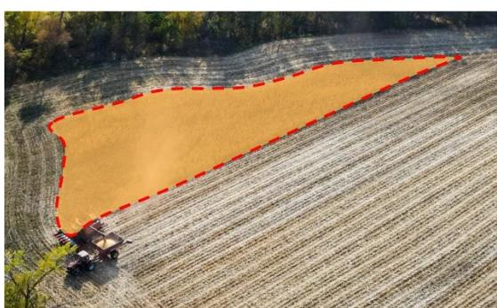
Select "Vehicle" in the menu. Select the settings and then press **ENTER** to start measuring. Drive around the perimeter of the plot of land and thereby its area will be calculated automatically.
