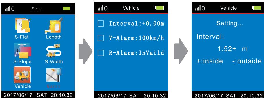
**Interval**      "–": without the width of the vehicle; "+": with the width of the vehicle.
